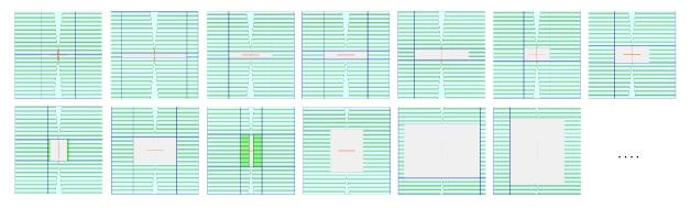
**Figure 1** Example apertures which are commonly employed to empirically determine an array of Area Output Factors (AOF). The AOF is a basic requirement for the machine-specific commissioning of the IQM calculation algorithm.
