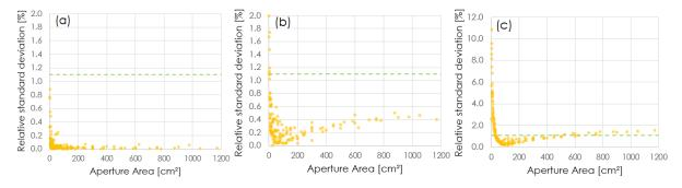
**Figure 3** Standard deviations (SD<sub>AOF</sub>) between IQM signals for a set of rectangular fields (AOF) relative to the referring average signal, measured at: (a) the same Linac with the same detector on the same day, (b) two matched Linacs with different chambers, (c) nine unmatched Linacs with different detectors. The single-machine single-session tolerance of 1.1% for SD<sub>AOF</sub> is represented by the green, dashed line.
